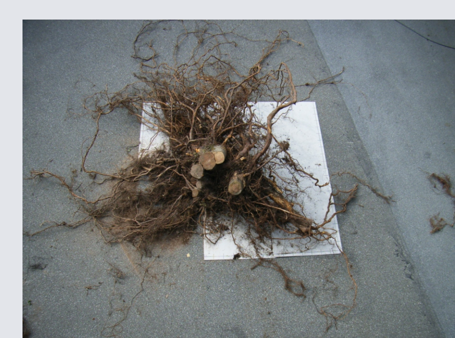
Figure 12: Isolated root collective ( Alnus incana L., rooted plants, and Salix daphnoides Vill., cuttings) from a hedge brush layer, 20 years old (rooting depth: 130 cm, total diameter: 800 cm)
