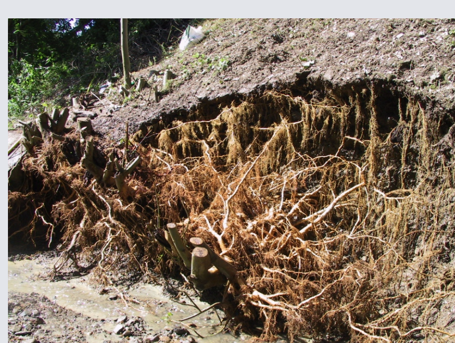
Figure 11: Isolated root collective ( Fraxinus excelsior L., rooted plants) from a slope grid, 25 years old (rooting depth: 130 cm, horizontal root extension: >200 cm)
